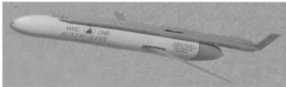
Fig. 4. SLOCUM glider in operation, shown is the prototype version with thermal engine mounted on top of the hull.
